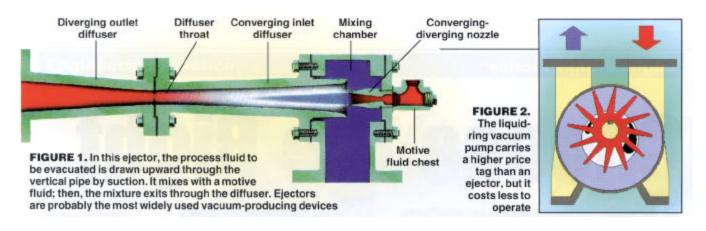
and chemical, plastics, pharmaceuticals and synthetic fibers plants; refrigeration at pulp and paper mills; drying in chemical and pharmaceutical plants; drying, flash cooling and refrigeration at food plants; and product degassing in steel mills. A related widespread use is condenser air venting at power plants.
