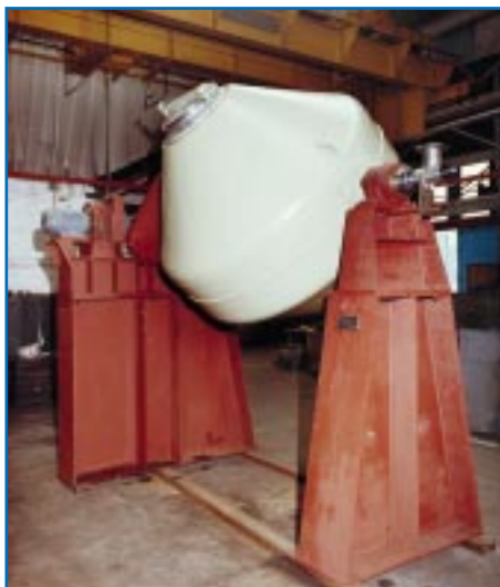
Figure 4. Double cone vacuum dryer Photo courtesy of Mitchell Dryers Limited, Carlisle, England
