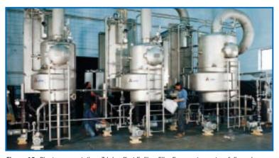
**Figure 13.** Plant representation. Triple-effect Falling Film Evaporator system followed by a double-effect forced circulation tubular finisher. A distillation essence recovery system was provided to recover the key essence components from the juice and in particular the methyl anthranilate.
