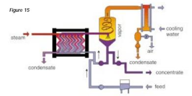
For most duties the conventional gasketed plate heat exchanger is specified. However for duties where the process fluid could attack the gasket, APV can offer the welded plate pair exchanger which eliminates elastomer gaskets on the process side.
