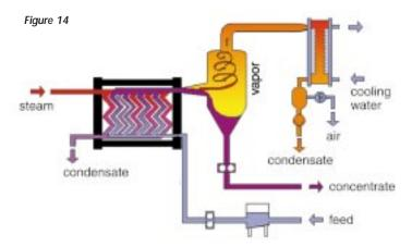
A clear advantage when processing temperature sensitive products is gained with a Paravap because most duties do not require liquid recirculation.
