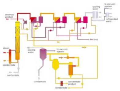
Figure 33. Flow diagram. Concord grape juice is extremely difficult to process due to the precipitation of tartrates during concentration. To keep temperatures above crystallization, as the grape juice is concentrated, a reverse feed design was selected, with dilute juice being directed to the low temperature effect first and leaving at the high temperature effect.
