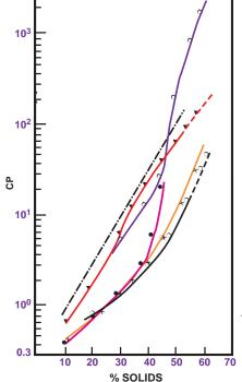
This waste water also varies from plant to plant, and the concentrate properties are extremely dependent on the feedstock. The product viscosity Figure 27) is plotted against % solids for different types of feedstock. In some cases there is a tenfold difference in viscosity.
