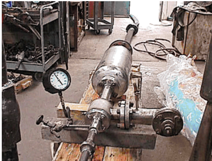
A typical ejectors is tested with a silencer for pressure drop and noise reduction.
